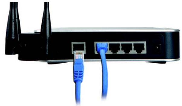
Figure 5-3: Connect the Internet
